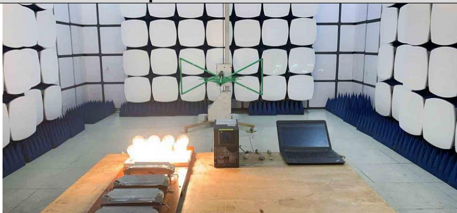
Set-up for Radiated Emission
